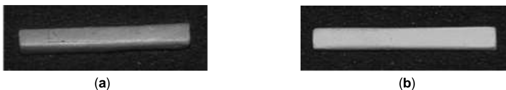
Figure 1. Extraction bars. ER bar (a), ER-MTK10 bar in composition of 70% ER and 30% MTK10 (b). Dimensions: 20 mm length and 3 \times 3 \text{ mm} of each side.
