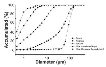
Figure 2: Curves of particle size distribution of the raw materials: quartz, bauxite, reprecipitated aluminum hydroxide, Bayer aluminium hydroxide, and alumina.
