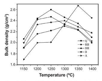
Figure 3: Values of bulk density as a function of sintering temperature for compositions Q (quartz), RH (reprecipitated aluminium hydroxide), BH (Bayer aluminium hydroxide), B (refractory bauxite) and A (alumina).
