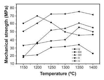
Figure 9: Mechanical strength versus sintering temperature for compositions: Q (quartz), B (refractory bauxite); RH (reprecipitated aluminium hydroxide); BH (Bayer aluminium hydroxide); and A (alumina).
