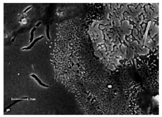
Figure 7: SEM micrograph of composition BH (Bayer aluminium hydroxide) showing agglomerated alumina.
