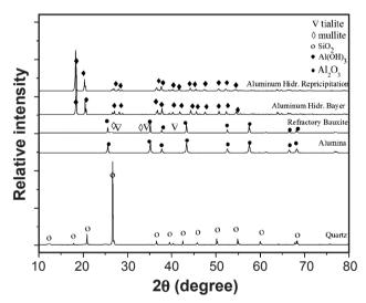
Figure 1: X-ray diffraction patterns of the raw materials. [Figura 1: Diffratogramas de raios X das matérias-primas.]
