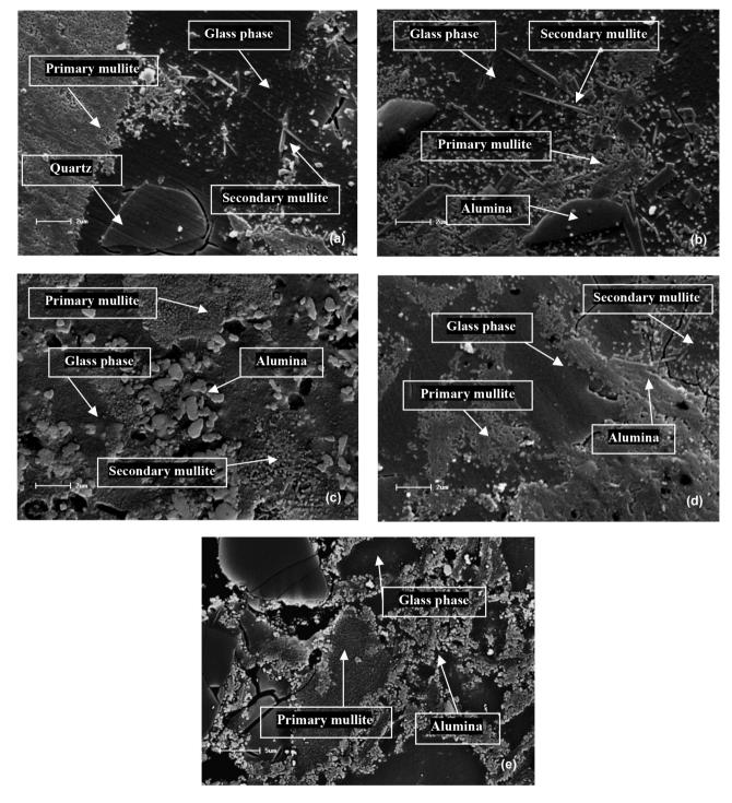
Figure 6: SEM micrographs of porcelain compositions sintered at 1300 °C: (a) Q (quartz), (b) B (refractory bauxite), (c) RH (reprecipitated aluminium hydroxide), (d) BH (Bayer aluminium hydroxide), and (e) A (alumina).
