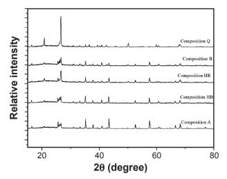
Figure 10: XRD patterns for compositions that presented higher mechanical strength for compositions: Q (quartz), B (refractory bauxite); RH (reprecipitated aluminium hydroxide); BH (Bayer aluminium hydroxide); and A (alumina).
