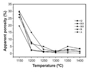
Figure 4: Apparent porosity as a function of sintering temperature for compositions Q (quartz), RH (reprecipitated aluminium hydroxide), BH (Bayer aluminium hydroxide), B (refractory bauxite) and A (alumina).
