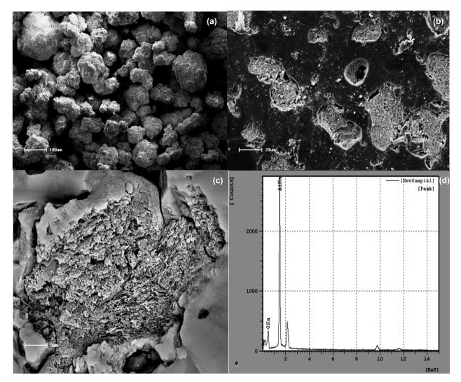
Figure 8: SEM micrographs of (a) Bayer aluminium hydroxide raw material, (b) BH (Bayer aluminium hydroxide), (c) lighter region in the microstructure, and (d) micro-analysis (EDS) of the lighter region.
