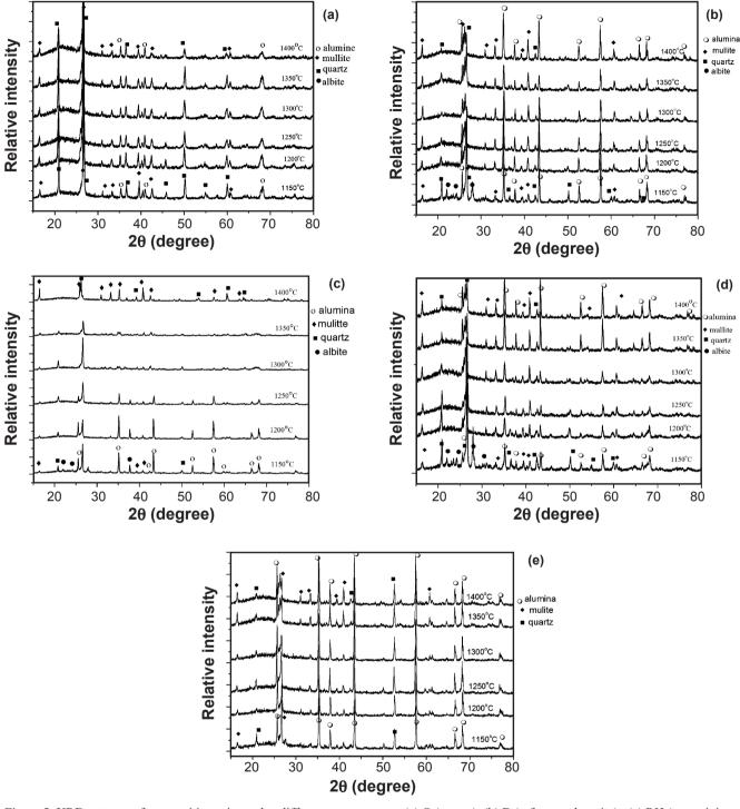
Figure 5: XRD patterns of compositions sintered at different temperatures: (a) Q (quartz), (b) B (refractory bauxite), (c) RH (reprecipitated aluminium hydroxide), (d) BH (Bayer aluminium hydroxide), and (e) A (alumina).
