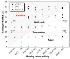
Figure 8. The relationship between rolling conditions and surface red degree value  $a^*$ .
