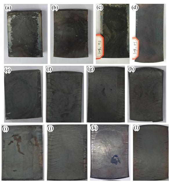
**Figure 3.** Surface morphology of oxide scale of samples after rolling. (a) 850°C-300s-5%; (b) 850°C-300s-20%; (c) 900°C-0s-10%; (d) 900°C-0s-30%. (e) 950°C-60s-10%; (f) 950°C-60s-20%; (g) 950°C-60s-30%; (h) 950°C-60s-40%. (i) 1000°C-6s-10%; (j) 1000°C-6s-20%; (k) 1000°C-6s-30%; (l) 1000°C-6s-40%.
