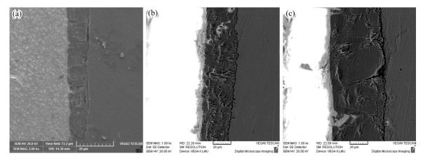
Figure 4. SEM of cross section oxide scale of rolled samples. (a) 850°C-6s-20%; (b) 950°C-60s-30%; (c) 1000°C-6s-40%.
