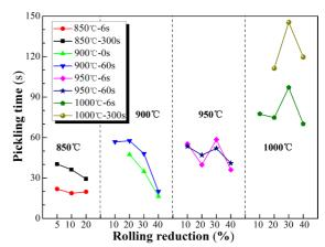
Figure 6. The pickling time of steel strip samples in different rolling conditions.
