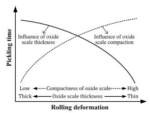
Figure 7. Schematic diagram of the effects of rolling deformation on the pickling time.
