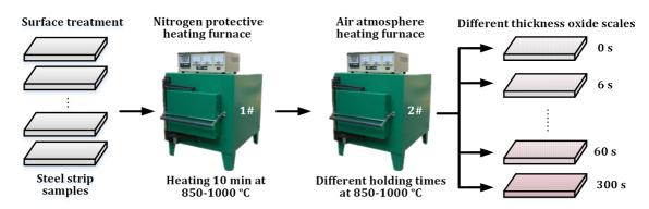
Figure 1. Sketch diagram of the oxide scales preparation.
