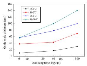
Figure 2. Thickness of oxide scales of steel strip in different heat processes.
