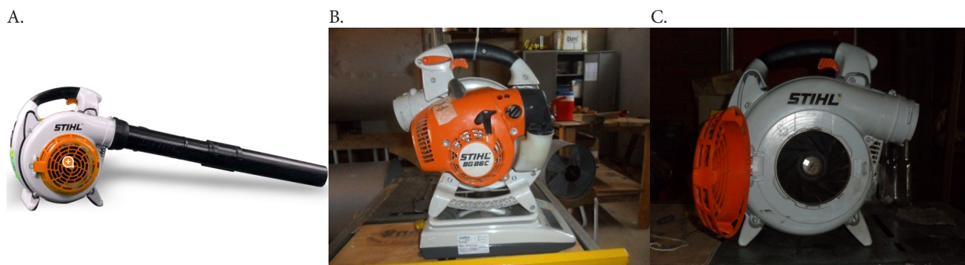
Figure 1. Air blower: (A) complete set, (B) with scale and (C) opened rotor
