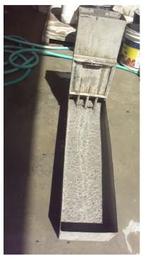
Figure 2. L-Box test in laboratory.
