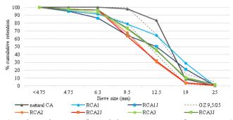
Figure 3. Granulometric curves of recycled coarse aggregates from sources 1, 2 and 3.
