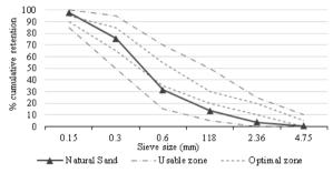
Figure 1. Granulometric curve of the natural fine quartz aggregate.
