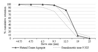
Figure 2. Granulometric curve of the natural coarse basaltic aggregate.
