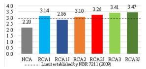
Figure 4. Shape index of the natural and recycled coarse aggregates from sources 1, 2 and 3, before and after jigging.
