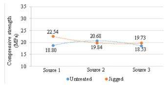
Figure 10. Effect of the source-treatment interaction in axial compressive strength.
