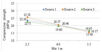
Figure 11. Effect of the mix-source interaction in axial compressive strength.
