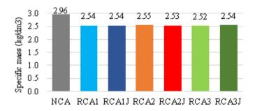
Figure 5. Specific mass of the recycled coarse aggregates from sources 1, 2 and 3.
