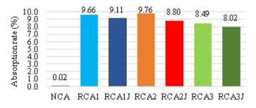
Figure 7. Absorption rate of the natural and recycled coarse aggregates
