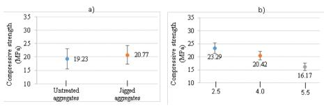
Figure 9. Isolated effects in axial compressive strength.
