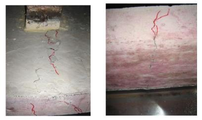
Figure 18. Beam V1A rupture configuration.
