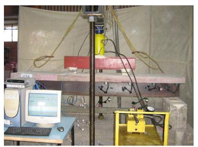
Figure 13. Test scheme for bending composite beam.
