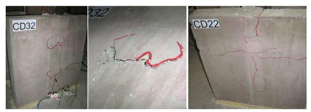
Figure 17. Cracks on push-out models' slab.
