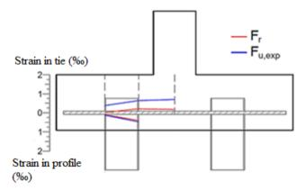
Figure 15. Strain in tie and profile of the BEmb20sch model.
