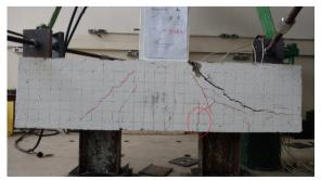
Figure 7. Failure plane of the BEmb10sch model.
