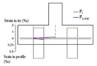
Figure 16. Strain in tie and profile of the BEmb30sch model.
