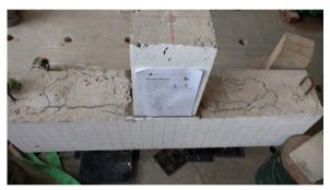
Figure 10. Cracks observed at the top of the model BEmb30sch.
