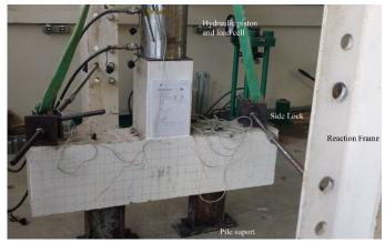
Figure 6. Test-system configuration.
