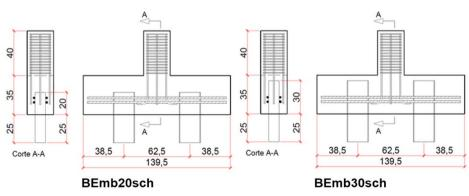
Figure 3. Models BEmb20sch and BEmb30sch (dimensions in cm)
