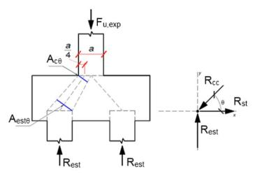
Figure 1. Strut and tie model proposed by Blévot and Frémy [2].
