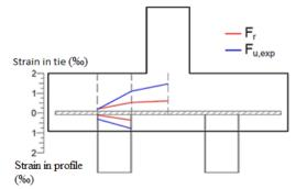
Figure 13. Strain in tie and profile of the BEmb10sch model.
