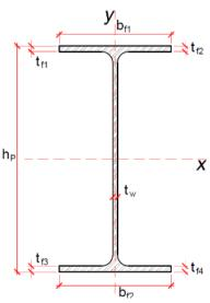
Figure 4. Cross section dimensions of steel profiles
