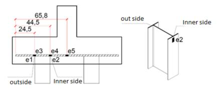
Figure 5. Position of extensometers on models.
