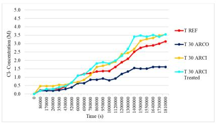
Figure 10. Chloride concentration in the anode compartment.
