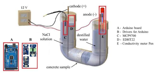
Figure 3. Scheme of chloride migration test adapted from Medeiros [45]
