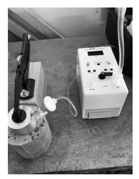
Figure 2. Porosiscope equipment.
