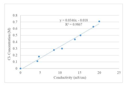
Figure 4. Calibration line between chloride concentration (M) and conductivity (mS /cm).
