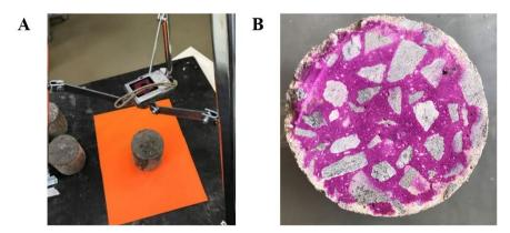
Figure 1. Test method of carbonation depth. A. Apparatus used to take the photographs. B. Specimen after spraying phenolphthalein.
