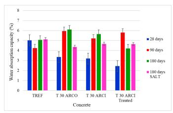
Figure 7. Results of water absorption capacity by immersion.
