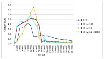
Figure 9. Monitoring of electrical current during chloride migration test.
