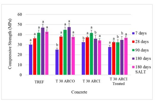
Figure 5. Results of resistance to axial compression.
