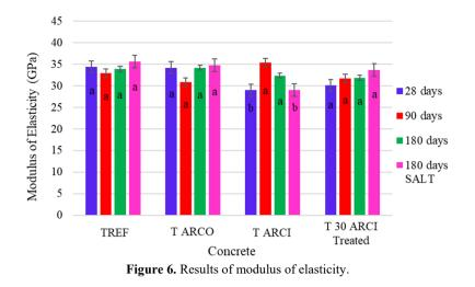
McGinnis et al. [2] pointed out a 26.4% reduction in the modulus of elasticity for concrete produced with 50% recycled aggregate, and a 34.4% decrease for concretes with a 100% substitution content. The reduction observed by McGinnis et al. [2] was higher than that obtained in this study, but this is justified by the fact that the researchers used a higher percentage of substitution of the natural aggregate than that used in this research.
