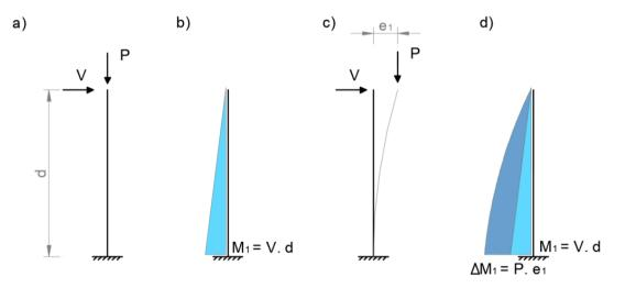
Figure 1. a) Cantilever beam. b) First-order internal forces. c) Beam displacement. d) Internal forces considering second-order effects.
