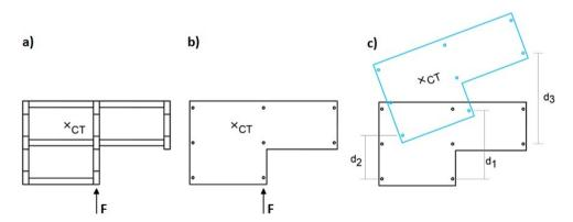
Figure 4. a) Force F at a building's floor with center of twist CT. b) Simplification of the building's floor. c) Structural elements presenting different eccentricities.
