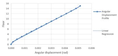
Figure 9. Angular displacement at each floor (building 4 and second analysis).
