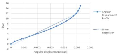
Figure 8. Angular displacement at each floor (building 4 and first analysis).
