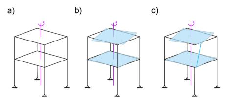
Figure 2. a) Torsional moment applied at a building. b) Rotation of the building's floor. c) Displacement of the highlighted column.
