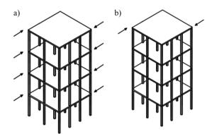
Figure 7. a) Distributed torsion couples. b) Single torsion couple.
