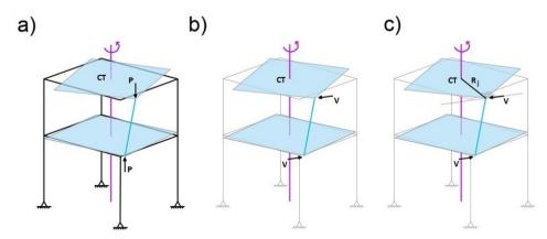
Figure 3. a) Eccentricity between vertical forces. b) Notional forces V. c) Distance R between the column and the CT.
