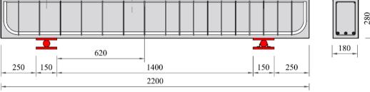
b) Side view and cross-section of the beams with shear reinforcement
