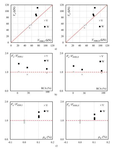
Figure 7 - Comparison between the experimental and theoretical for the tested beams.
