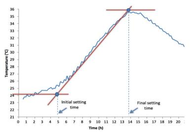
Figure 4. Scheme representing the determination of the initial and final setting times by the tangent method.
