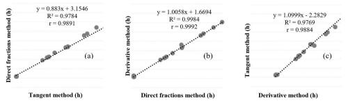
Figure 12. Correlation between the final setting times obtained by the tangent, direct fraction, and derivative methods.
