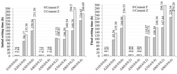
Figure 13. Initial and final setting times for mortars with cements F and Z, by the direct fraction method.
