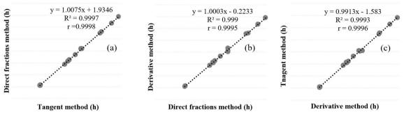
Figure 10. Correlation between the initial setting times obtained by the tangent, direct fraction, and derivatives methods, for mortars with cement F and cement Z.
