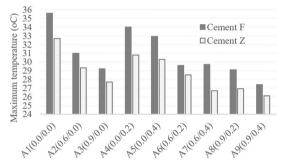
Figure 8. Maximum temperatures reached by mortars with cement F and cement Z.
