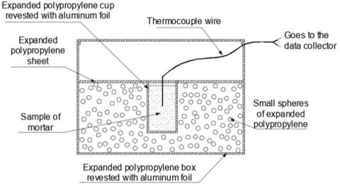
Figure 2. Scheme of the semi-adiabatic calorimeter in section.
