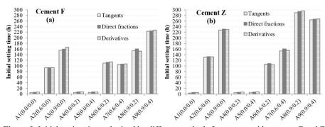
Figure 9. Initial setting times obtained by different methods for mortars with cements F and Z.
