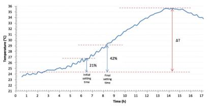
Figure 5. Scheme representing the determination of the initial and final setting times by the direct fraction method.
