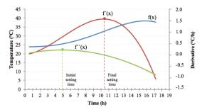
Figure 6. Scheme representing the determination of the initial and final setting times by the derivatives method.
