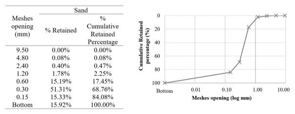
Figure 1. Particle size of Sand.
