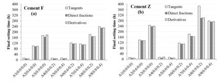
Figure 11. Final setting times obtained by different methods for mortars with cements F and Z.
