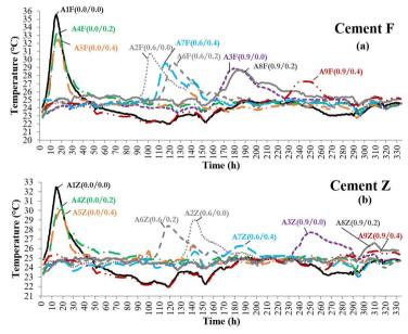
Figure 7. Evolution of the mortar temperatures over time, for cement F (a) and cement Z (b).
