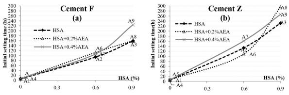
Figure 14. Effect of the increase in the content of HSA at the initial setting time of the mortar.
