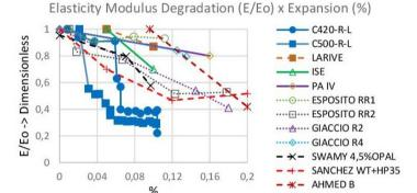
Figure 13. Elasticity modulus degradation of the concretes C420/500-R-L compared to several authors (see Table 2) (AUTHOR).
