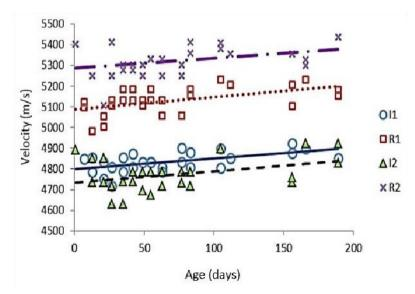
Figure 4. UPV vs. age in the concrete beams tested (see Table 1) [3].
