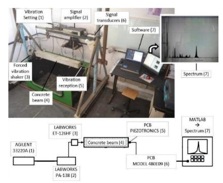
Figure 7. Scheme of the LRF test (modified of Barreto [3]).
