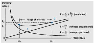
Figure 11. Proportional Damping Scheme [21].
