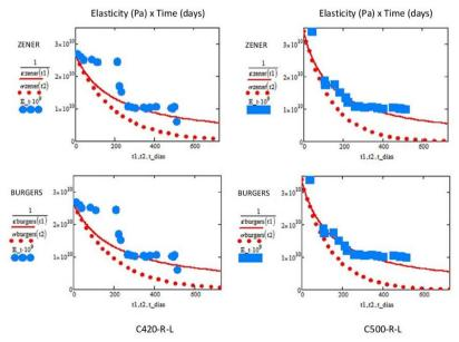
Figure 14. Elasticity modulus of the concretes C420/500-R-L; creep - continuous line; relaxation - dotted line; experimental - dot (AUTHOR).
