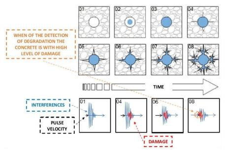
Figure 5. Illustration of UPV test vs. damage by the growth of gel of AAR (AUTHOR/UFPB).
