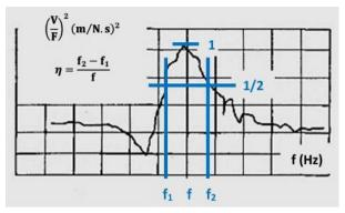
Figure 1. Schematic diagram for calculating the loss factor (adapted of Nagy [6]).
