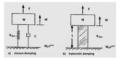
Figure 8. Damping for single degree of freedom: a) Viscous; b) Hysteresis (adapted of Nashif et al. [7]).
