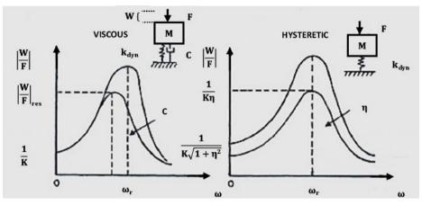
Figure 3. Dynamic response of viscous and hysteresis systems (adapted of Nashif et al. [7]).
