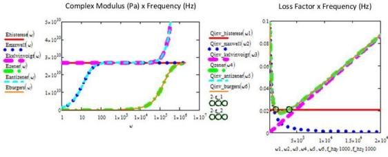
Figure 15. Complex modulus and attenuation curve (loss factor): concrete C420-R-L (AUTHOR).
