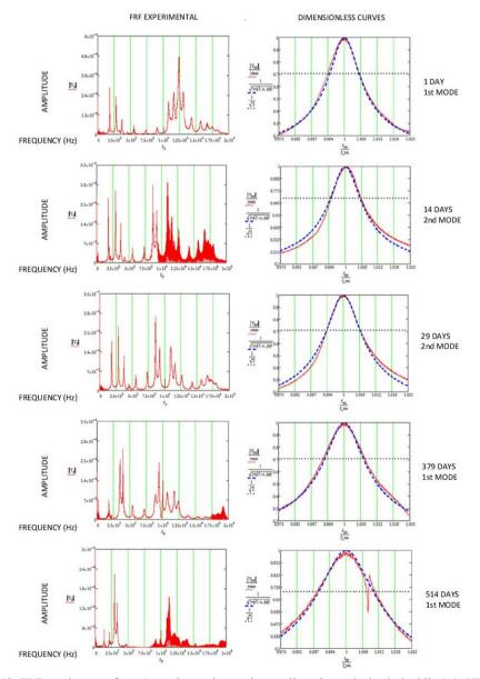
Figure 12. FRFs and curves for  $\eta$  (experimental - continuous line; theoretical - dashed line) (AUTHOR).
