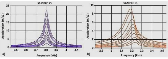
Figure 2. a) FRF to sample S3; b) FRF to sample S1 (adapted of Leśnicki et al. [2]).
